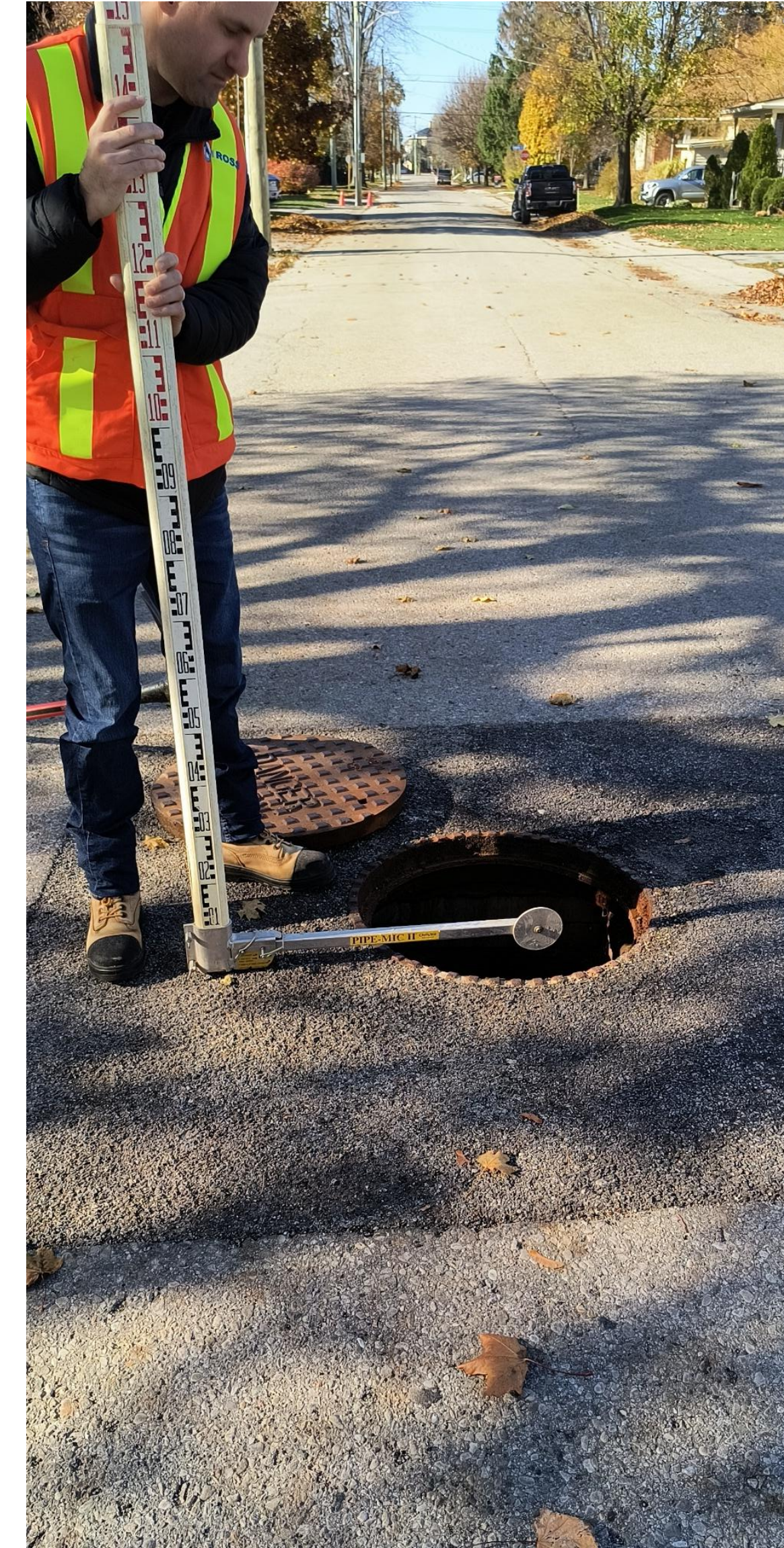
Pipe-Mic attachment to measure pipe dia.
